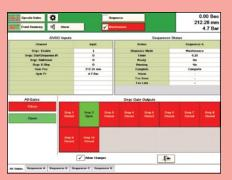
4. Press "Operate Gates" - "Allow Changes"\* Open/close valve gates (test)
